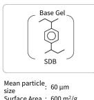
size . 00 µm Surface Area : 600 m²/g Pore volume : 1.1 mL/g Pore size : 70 Å PH range of use : 1 - 14 InertSep PLS 2 is a cartridge filled with styrene divinylbenzene polymer gel (SDB). It has a retention capacity greater than C18 and excellent stability in a wide pH range.
